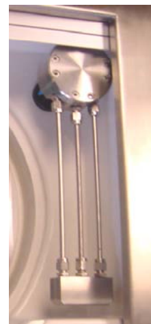
Water, detergent drying gas feed
